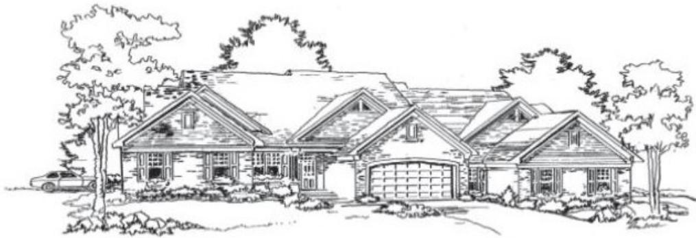
*Example of a triplex with a garage for each end unit, accessed from the side. The triplex design includes a number of techniques to provide architectural variety, with materials variety, multi-planned roofline, window treatments, and building modulation.*
